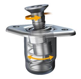
The materials specified for the components are common aerospace alloys, such as A-286, 17-4 PH, AISI 4140/ 4130, and titanium alloys. For special applications, the nut plates could be manufactured from ceramics or composite materials. Enduralock can offer the technology in all commonly used industry thread sizes (.1900-32, .2500-28, .3125-24, .3750-24, .4375-20 and .5000-20).
